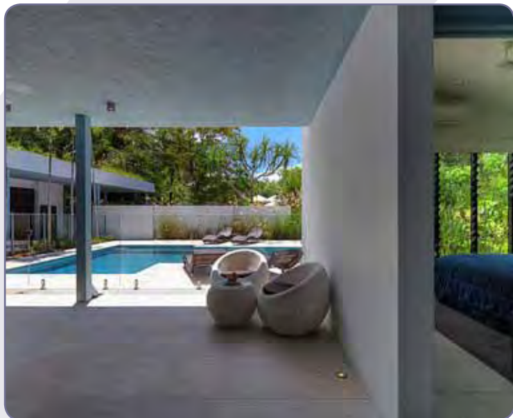
Heavier mass homes can work well if well shaded and light coloured Chris Vandyke Designs. Photo: Sean Reason
